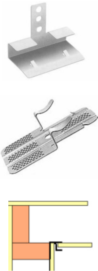
Two-stud corners with drywall clips use the least wood and give the best thermal performance.
