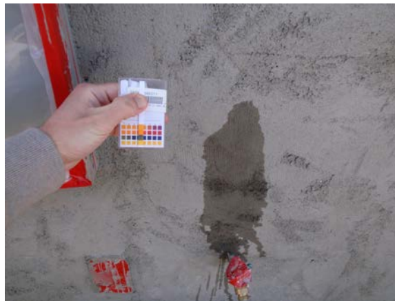
Figure 24. pH testing of the base coat
