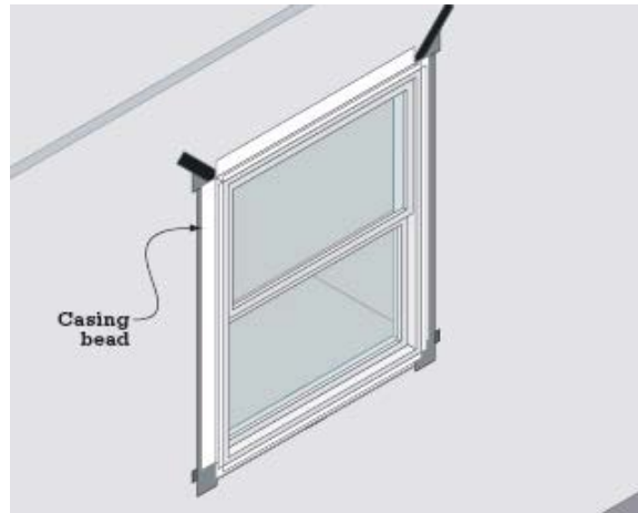
Figure 12. Detail of casing bead installed against a window (Courtesy of BuildIQ)
