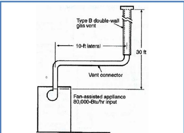
**Figure 2. Fan-assisted appliance**
