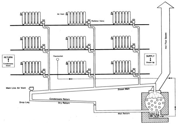
Figure 3. Schematic of one-pipe gravity return steam system
