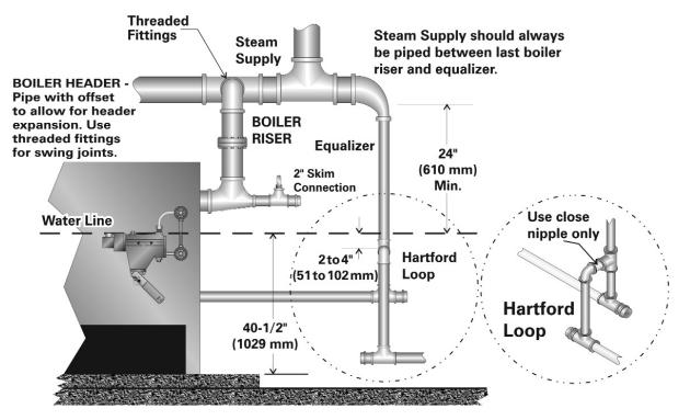
Figure 7. Specifications for how to pipe a Series 211A<sup>™</sup> natural gas steam boiler by Peerless<sup>®</sup> Boilers
