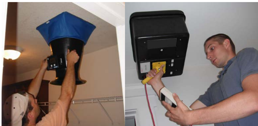
Figure 2. Measuring exhaust flow with a flow hood and exhaust fan meter
