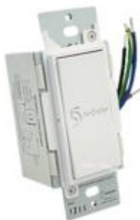
Figure 11. Many timer controls can be programmed to cycle fans on and off. For an equivalent 30 CFM continuously, a 50-CFM fan can operate 36 minutes per hour. The fan can also be controlled on-demand.
