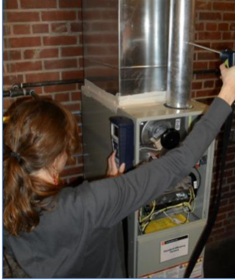
Figure 4. Draft pressure testing using combustion analyzer
