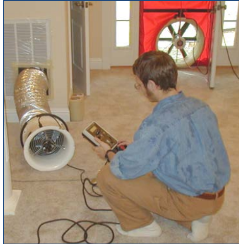
Figure 2. Duct pressurization test
