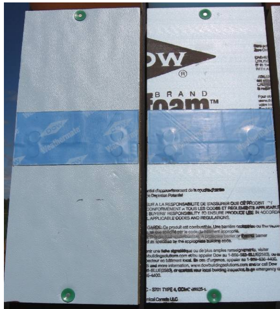
Figure 35. Dow Weathermate butyl on ffPIC (left) and XPS (right)
