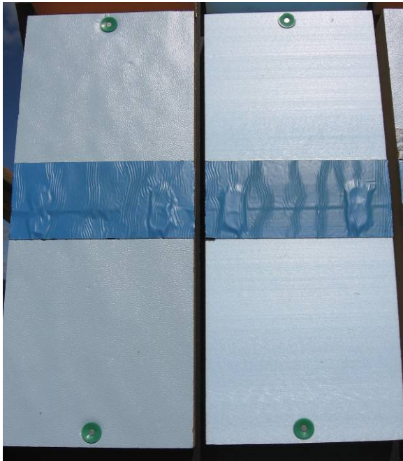
Figure 24. Henry Blueskin on ffPIC (left) and XPS (right)
