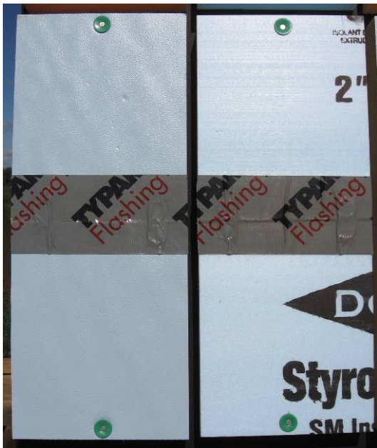
Figure 21. Typar tape on ffPIC (left) and XPS (right)
