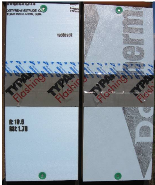
Figure 22. Typar tape with termination tape on ffPIC (right) and XPS (left)
