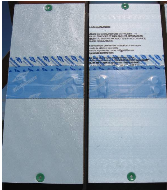
Figure 33. Dow Weathermate butyl with termination tape on ffPIC (left) and XPS (right)
