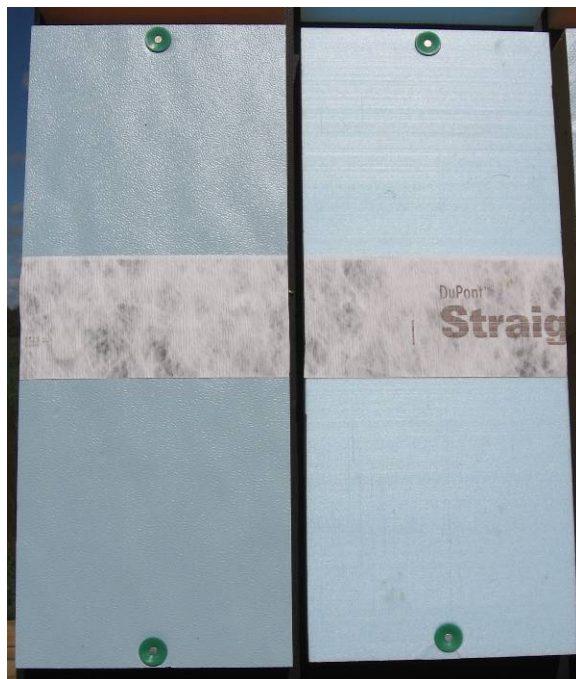
Figure 31. DuPont Straightflash tape on ffPIC (left) and XPS (right)
