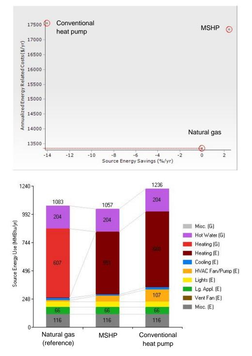
Figure 7. BEopt output comparing natural gas, MSHPs, and conventional heat pump—New York
