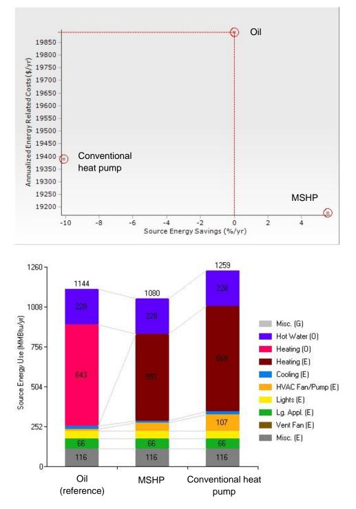
Figure 5. BEopt output comparing oil, MSHPs, and conventional heat pump-New York
