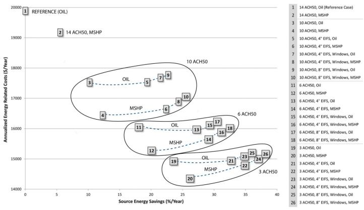
Figure 11. BEopt output comparing envelope improvements—air sealing
