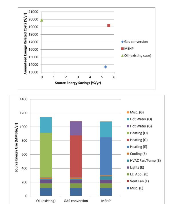
Figure 9. BEopt output for converting oil to natural gas or MSHPs—New York
