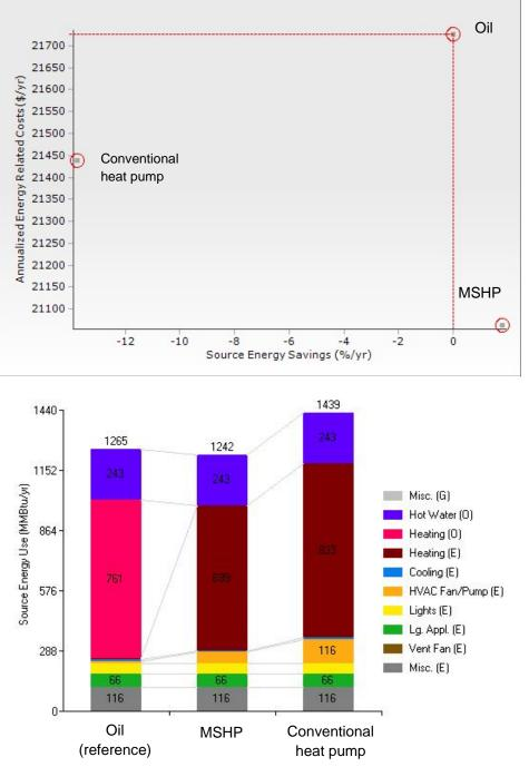
Figure 6. BEopt output comparing oil, MSHPs, and conventional heat pump—Boston
