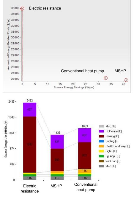
Figure 4. BEopt output comparing electric resistance, MSHPs, and conventional heat pumps—Boston
