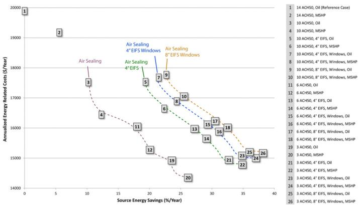
Figure 12. BEopt output comparing envelope improvements—insulation and windows
