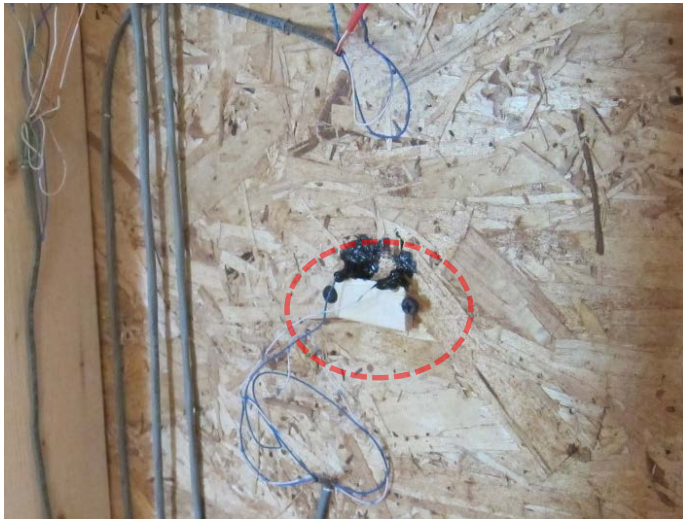
Figure 22. Sheathing-insulation interface wafer sensor location
