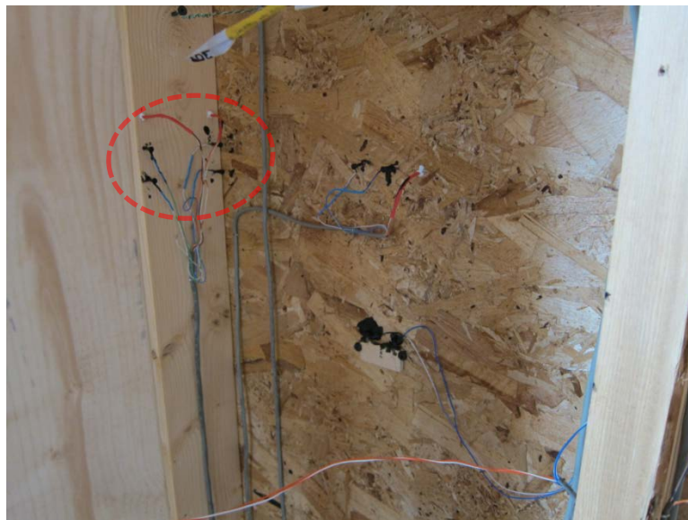
Figure 30. Framing MC/temperature sensor locations
