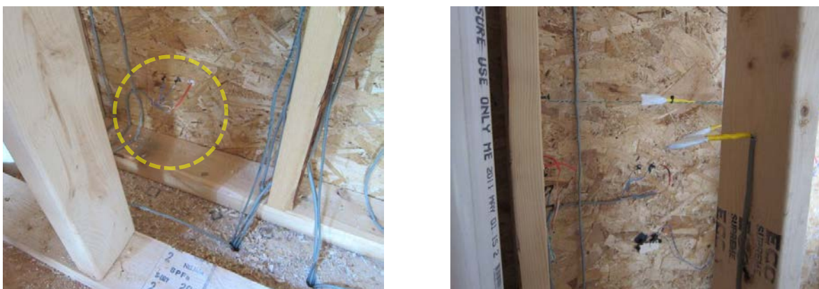
Figure 9. (L) Temperature and MC sensor at sheathing; (R) sensors at mid-height of stud bay
