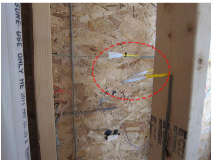
Figure 27. Stud bay cavity T/RH sensor locations
