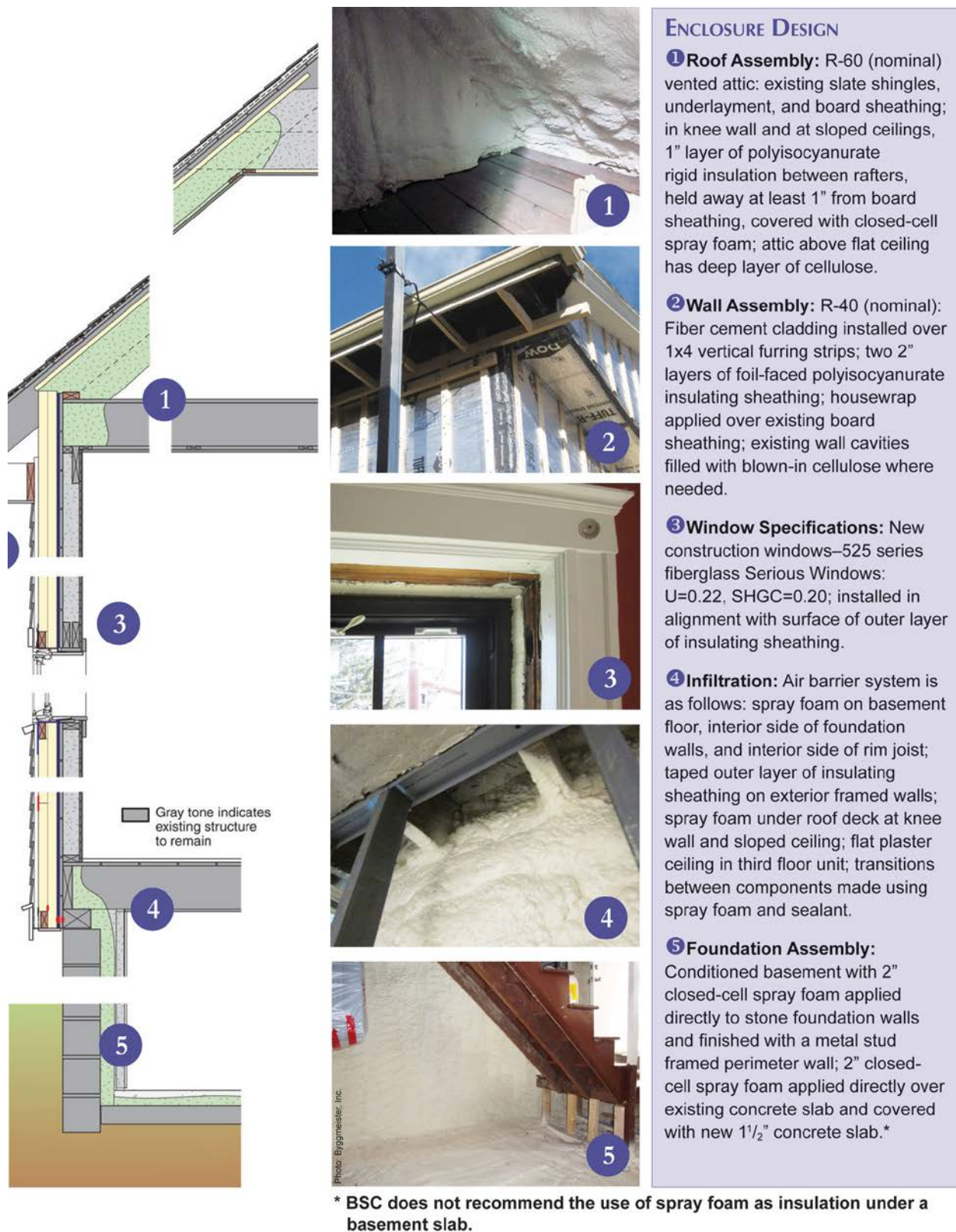
Figure A.8.2. Jamaica Plain DER Enclosure Profile
