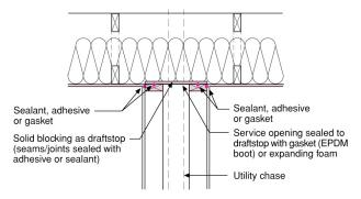
Flexible gasket sealed to top plate or other solid blocking allows movement of penetrating element without loosing the air seal Recessed ceiling fixtures in insulated ceiling should be both insulation contact ("IC")- and air tight rated. The housing of the recessed fixture should also be sealed (with caulk or an effective gasket) to the ceiling gypsum board.
