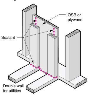
Solid draftstop material sealed to framing to isolate utility chase cavity
