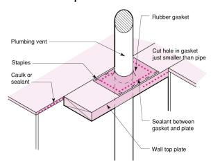
Flexible gasket sealed to top plate or other solid blocking allows movement of penetrating element without loosing the air seal
