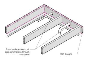
Penetrating pipes, conduits, ducts, projecting beams etc, are sealed to the air barrier element that they penetrate.
