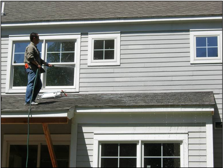
Figure 12: Spray wetting of the siding outside the test bay
