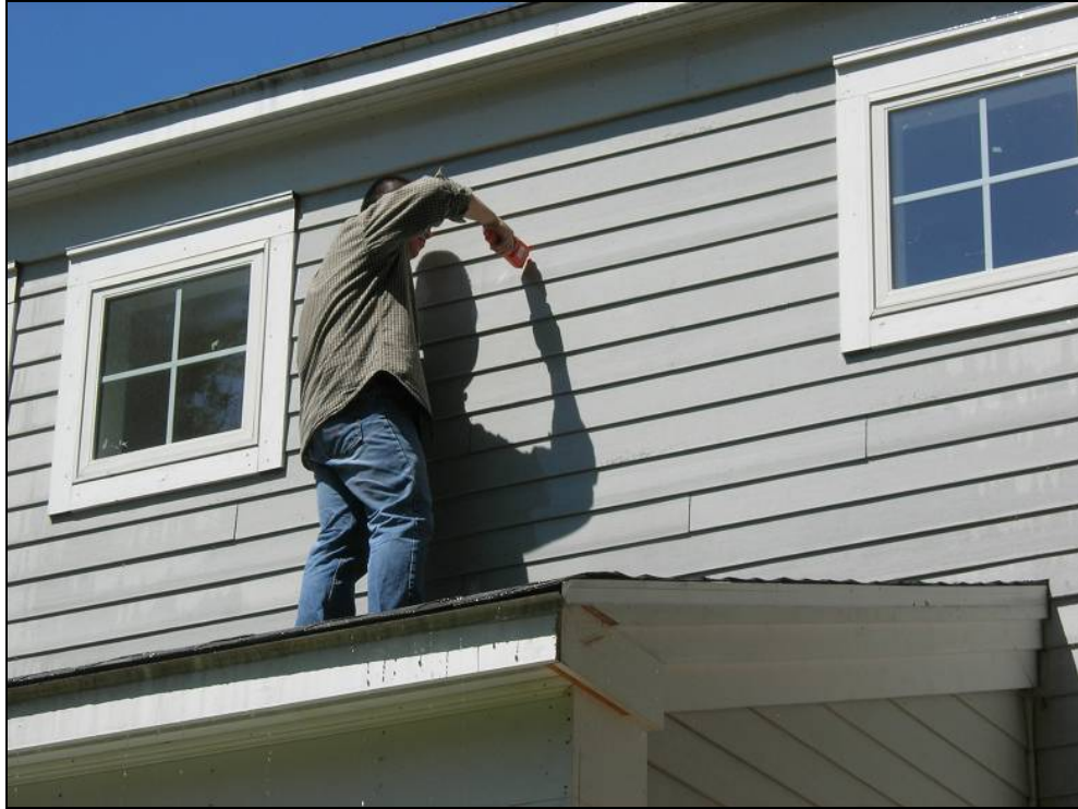
Figure 14 Testing the uniformity on the siding outside the test bay
