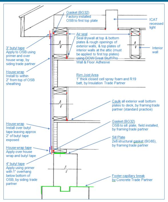
Figure 3. Enclosure air sealing specification detail.
