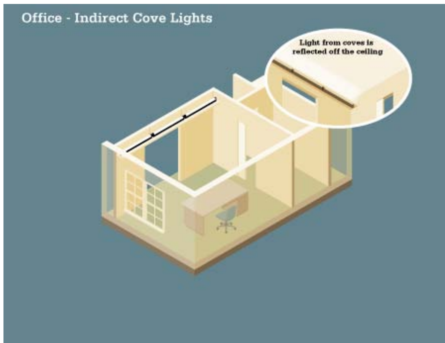
Figure 64. Indirect - cove lights. Light cove or valance, T-5 or T-8 strip lights, continuous.
