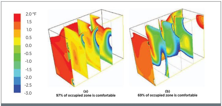
Figure 1. Plots of acceptable draft temperature in cooling mode when the room is supplied by  $55^{\circ}F$  (286 K) through 8-in. (0.2 m) × 4-in. (0.1 m) supply inlet: (a) supply velocity of 394 fpm (2 m/s) and (b) supply velocity 788 fpm (4 m/s). Figures by El Hassan Ridouane
