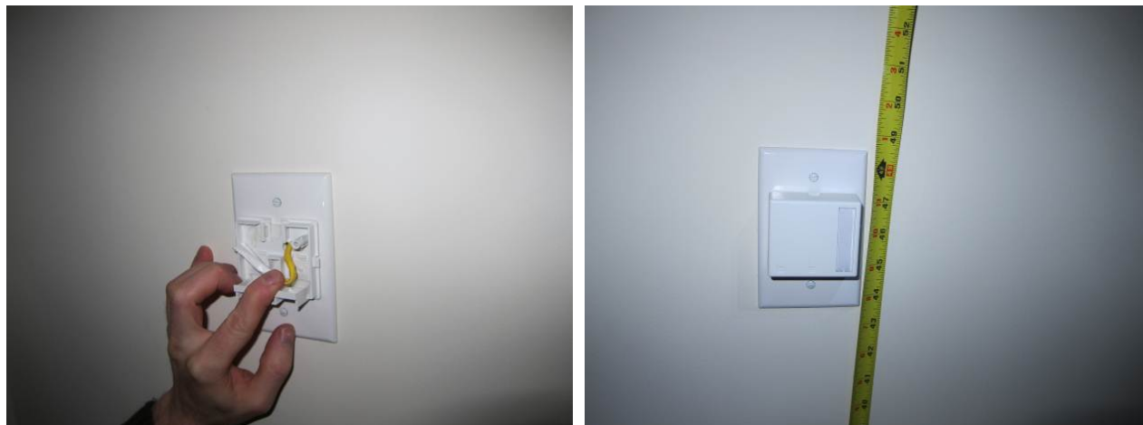
Figure 52. Sensor measure interior (bedroom) T/RH sensors
