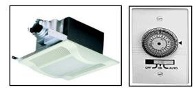
All three of these criteria can typically be achieved by installing one ENERGY STAR® bath fan. The fan can operate continuously or in conjunction with a timer control (such as the Grasslin pin-timer shown to the left). If on a timer, the fans should be also wired to allow occupants to turn the fan "On" from a manual switch within the bathroom. The timer then should be set-up to comply with the guidelines set forth by
