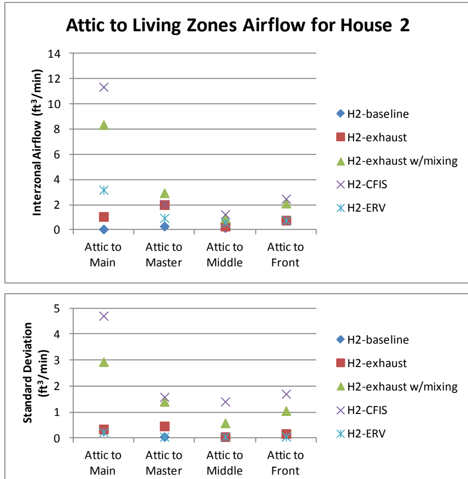
Figure 25. Airflow from attic to living area zones in House 2, for the baseline test and four different ventilation systems
