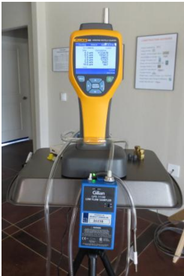
Figure 17. VOC sampling pump and solid sorbent sample tube; airborne particulate counter on top of sampling fixture
