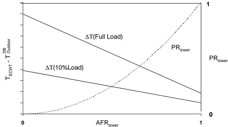
**Figure A3-4: Cooling Tower Fan Operation**
