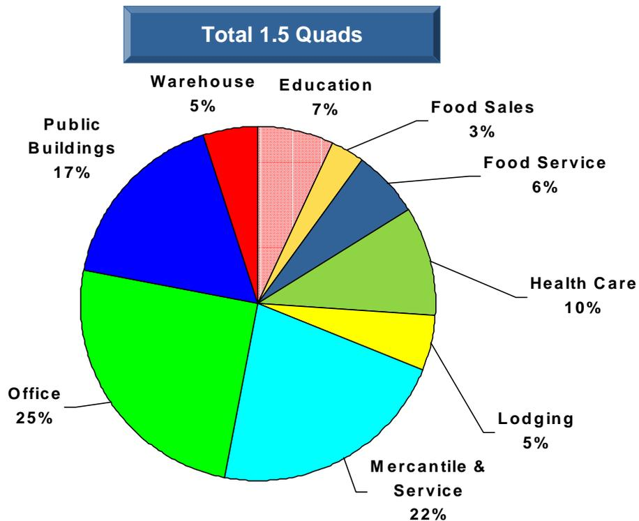
Figure 5-13: Parasitic Primary Energy Use - Building Type Breakdown
