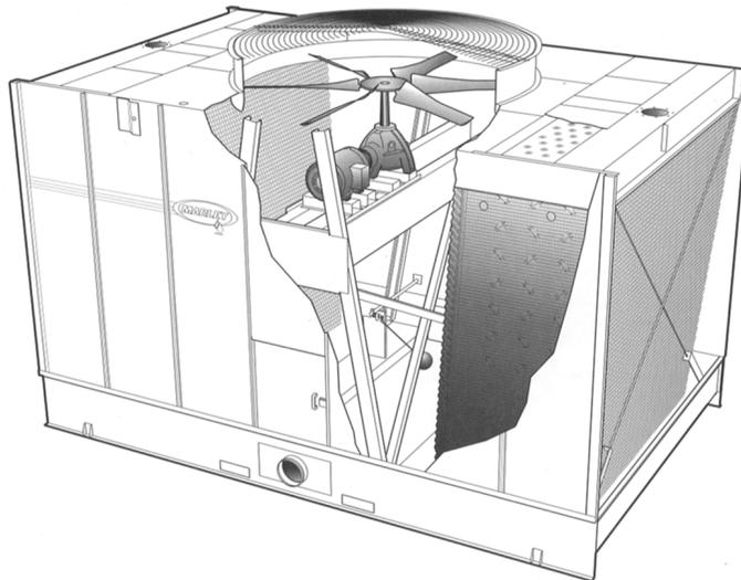
**Figure 3-13: A Cooling Tower With A Propeller Fan**
