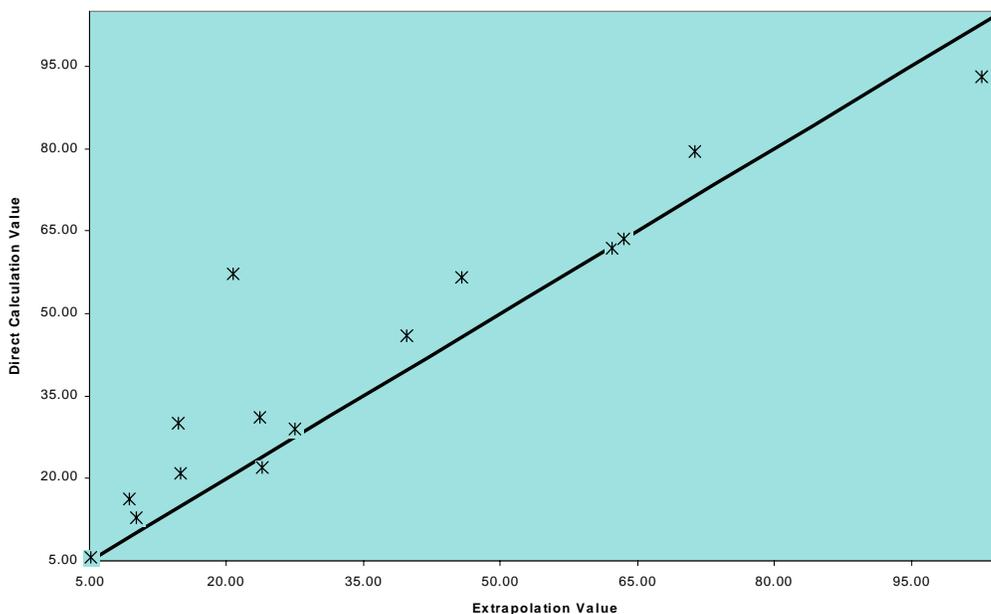
**Figure 5-11: EUI Extrapolation Data Comparison (Coil & Building Loads kBtu/h/SF)**
