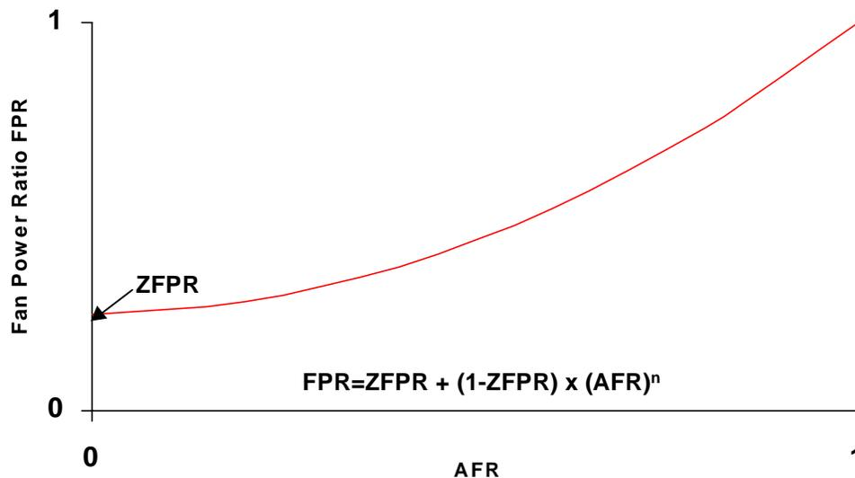
Figure A3-2: Fan Power Curve
