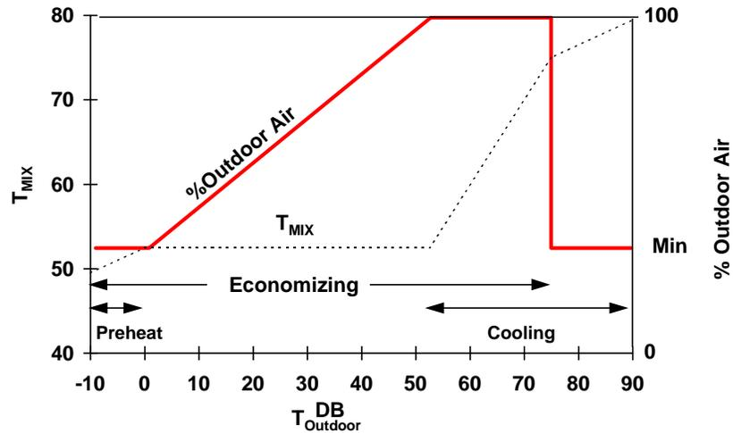
**Figure A3-3: Air Handling Unit Air Mixing**
