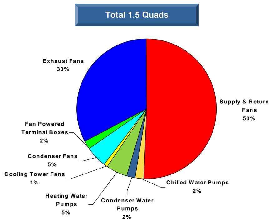
**Figure 1-1: Parasitic Primary Energy Use -- Equipment Breakdown**
