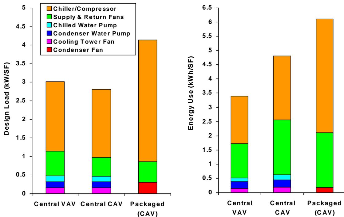
**Figure 1-5: Design Load and Energy Use Comparison of Central VAV, Central CAV and Packaged Systems**
