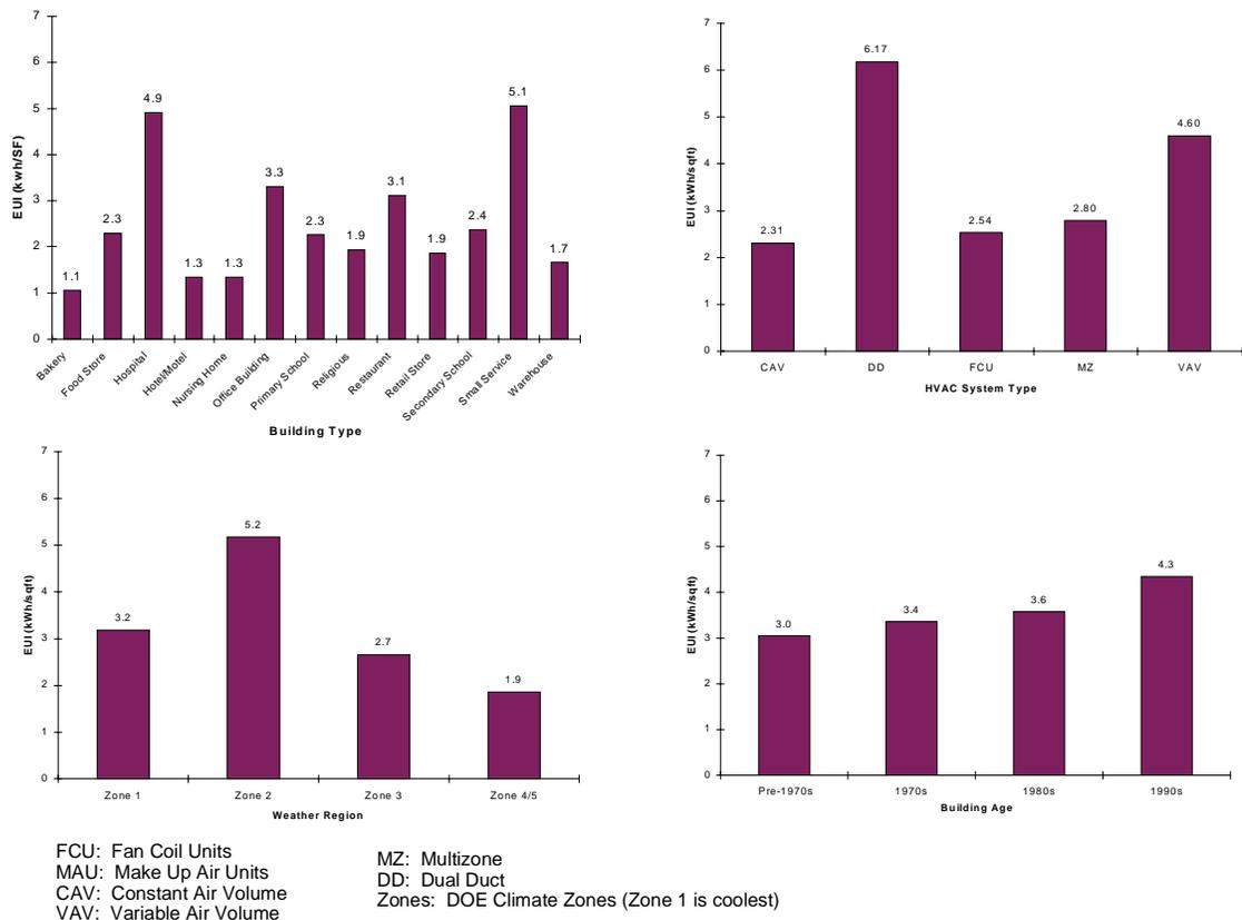
Figure A1-6: XenCAP™ Fan Power Data
