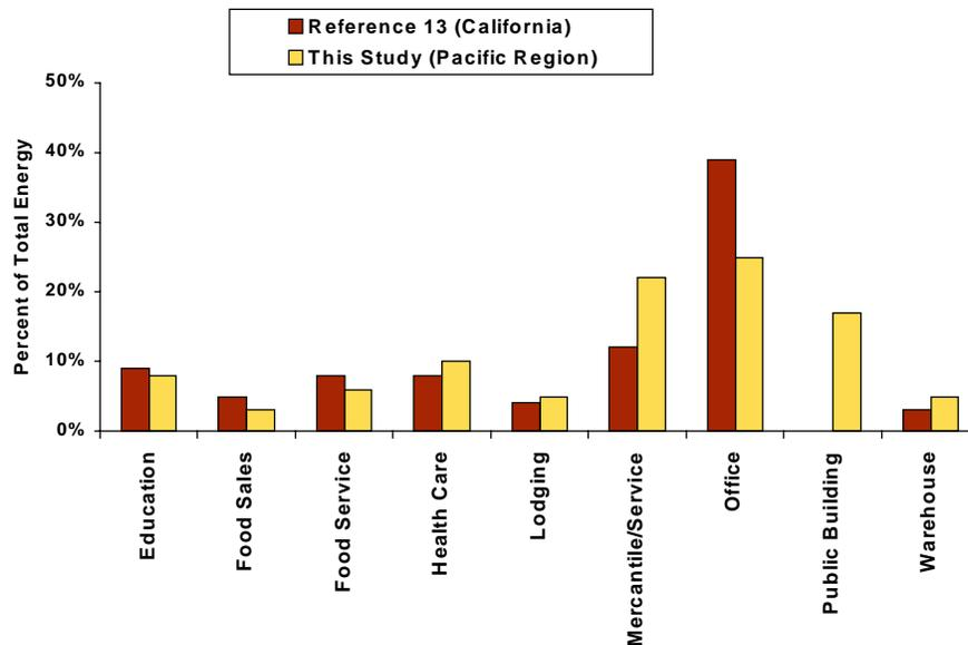
**Figure 5-19: Thermal Distribution Energy Use Breakdown by Building: Comparison to Reference 13**
