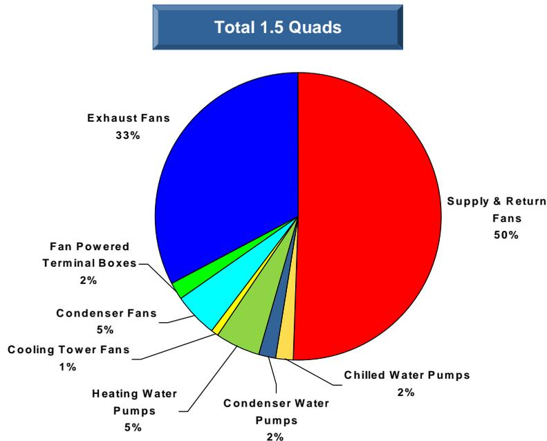
**Figure 5-12: Parasitic Primary Energy Use – Equipment Breakdown**
