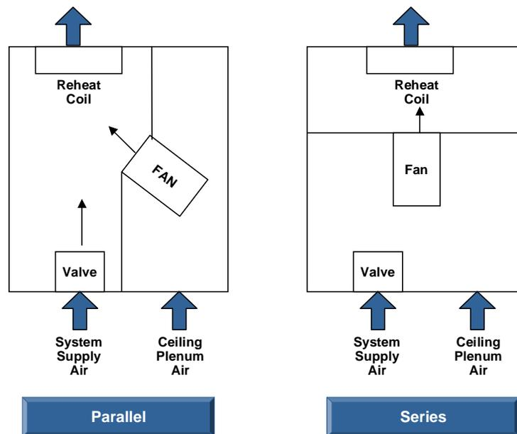
Figure 3-7: Parallel and Series Fan Boxes
