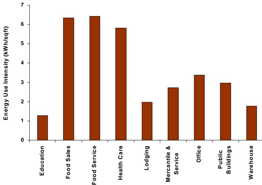
**Figure 5-14: Parasitic Site Energy Use Intensity by Building Type**
