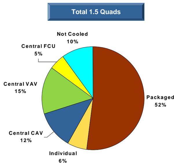
**Figure 5-16: Parasitic Energy Use - System Type Breakdown**
