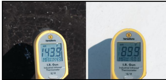
Figure 1: Dark vs. Cool Roof Surface Temperatures
