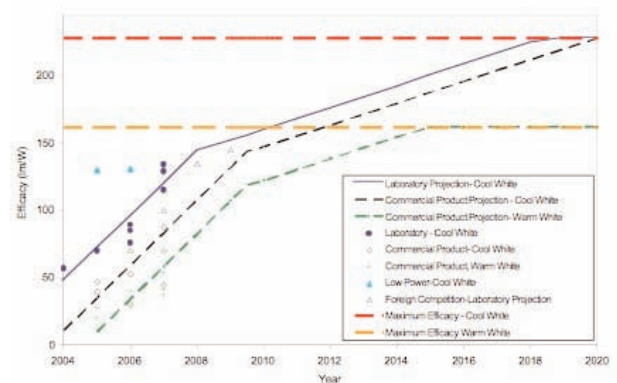
Figure 2-11 White Light LED Device Efficacy Targets, Laboratory and Commercial 41
