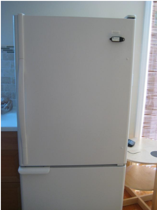
Figure 27. Installation of USB Track-It Data Logger
