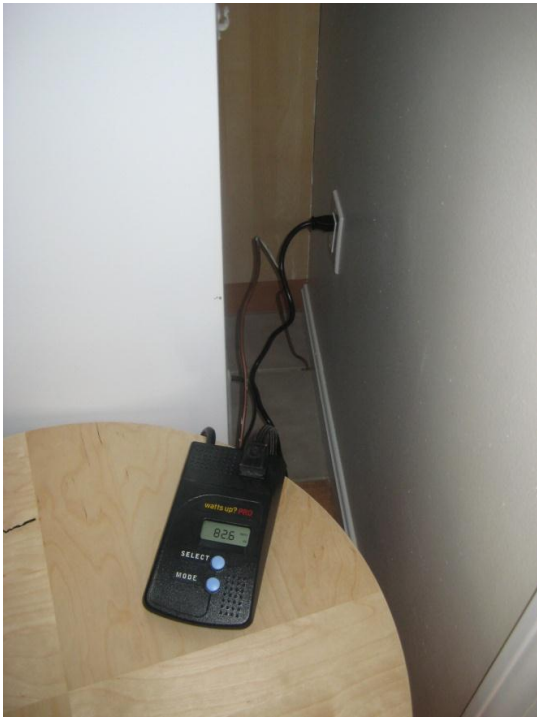
Figure 26. Installation of Watts Up Pro Power Meter
