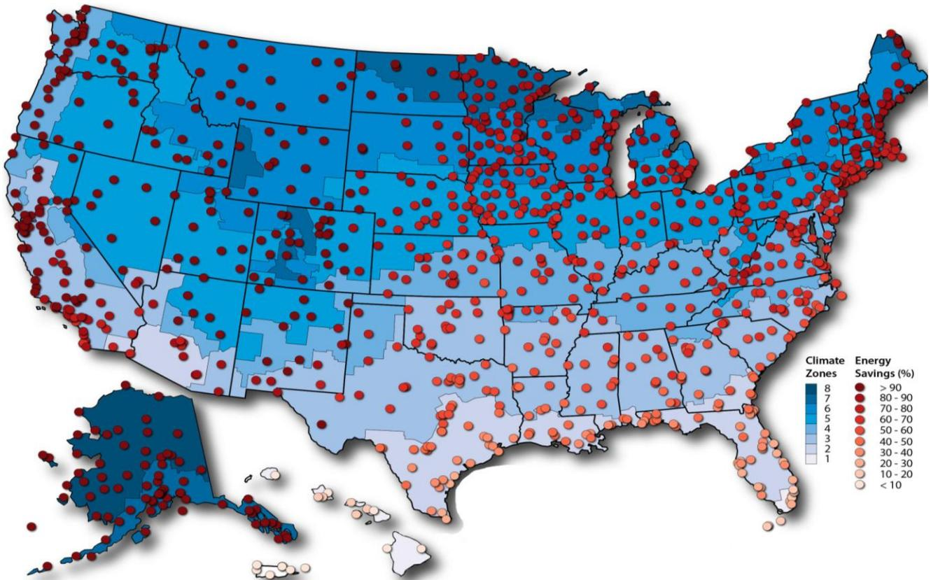
**Figure 4** Energy savings potential for recommended envelope, Stage 2: Economizer + Direct Evap. Cooling.<sup>15</sup>
