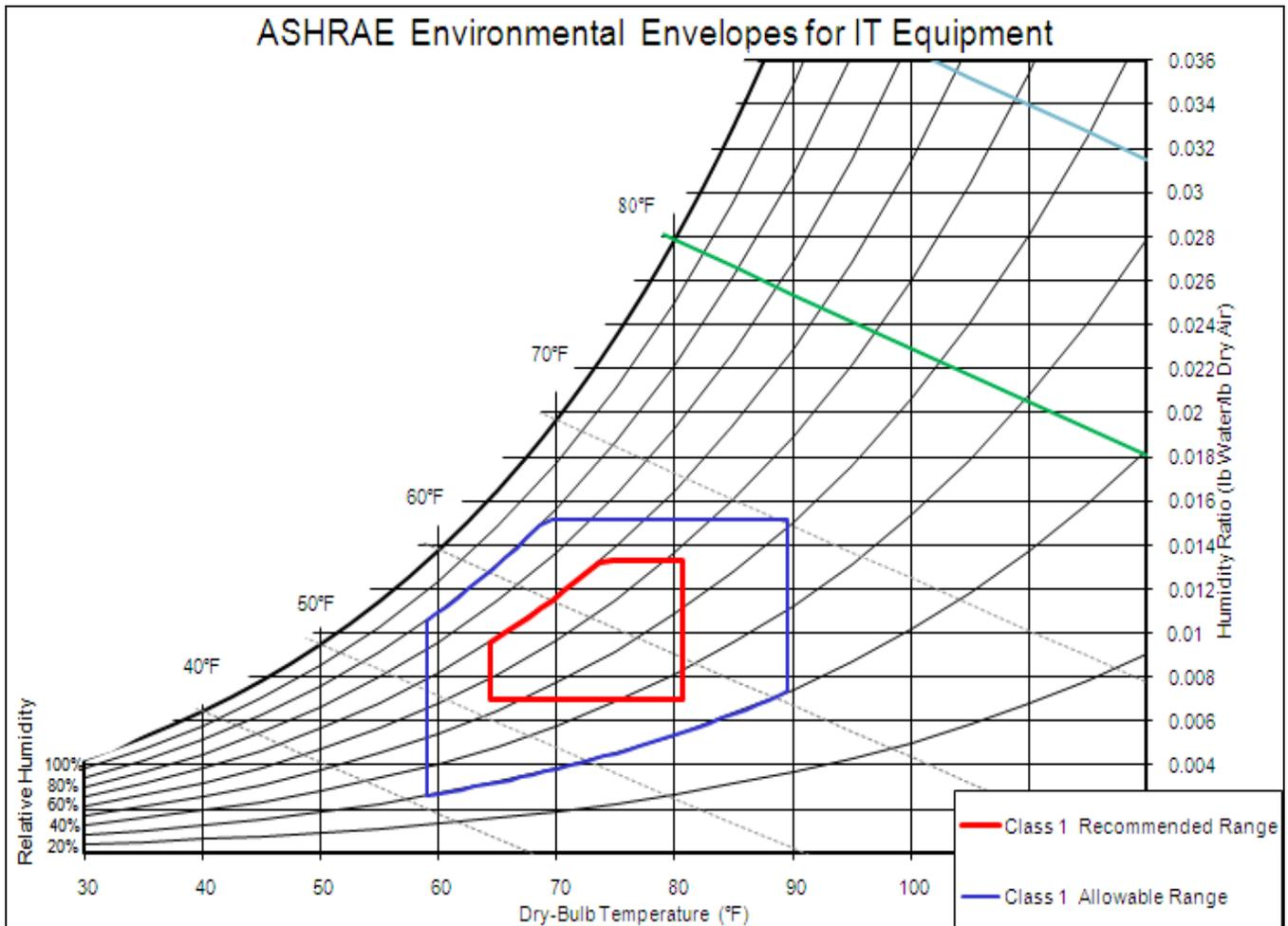
**Figure 1** Psychrometric chart showing ASHRAE recommended and allowable environmental envelopes for IT equipment.<sup>2</sup> (Source: Ian Metzger, NREL)
