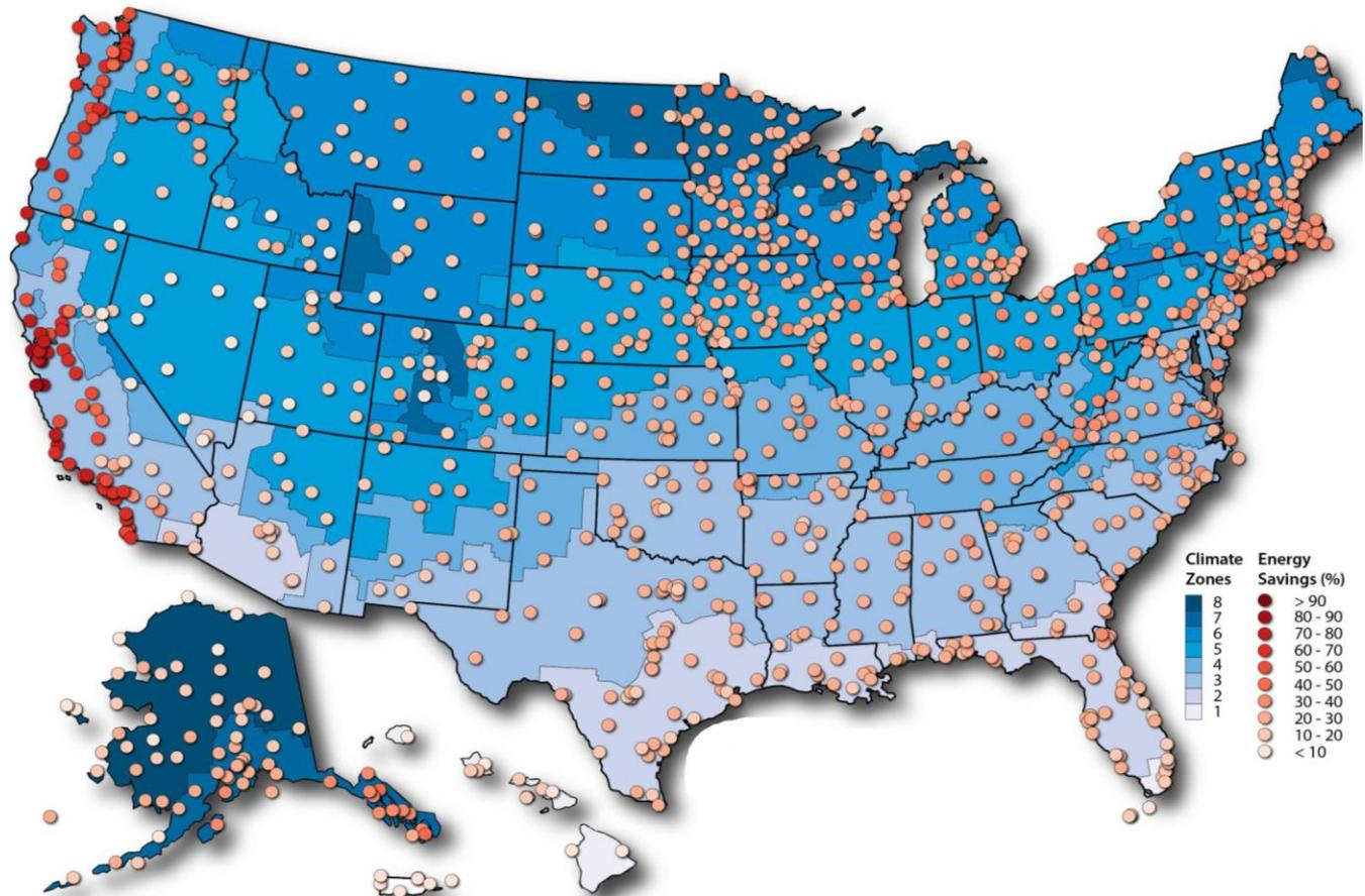
**Figure 3** Energy savings potential for recommended envelope, Stage 1: Economizer Cooling.<sup>15</sup> (Source: Billy Roberts, NREL)
