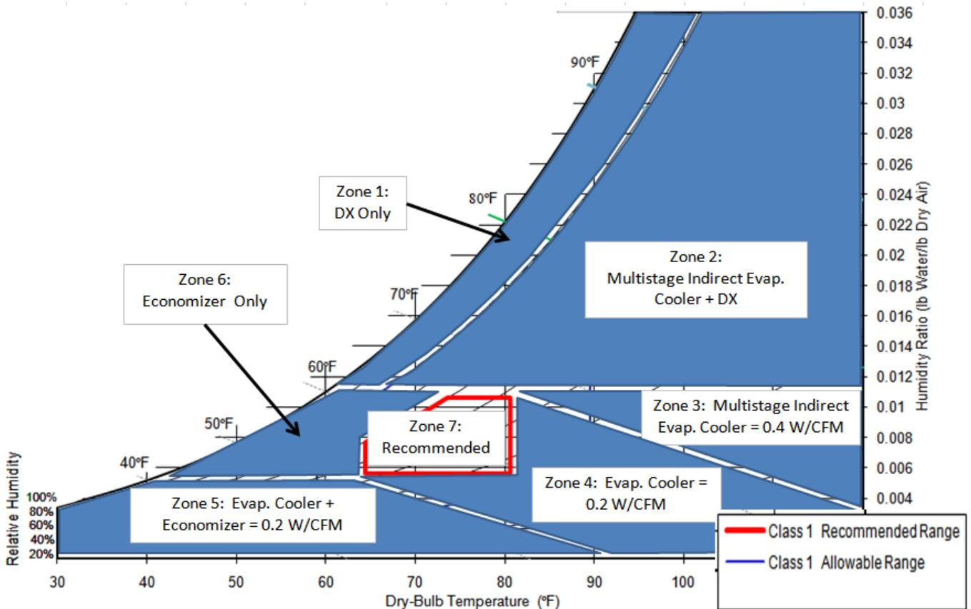
**Figure 2** Psychrometric chart displaying bin zones for the recommended envelope and alternative cooling strategies. (Source: Ian Metzger, NREL)
