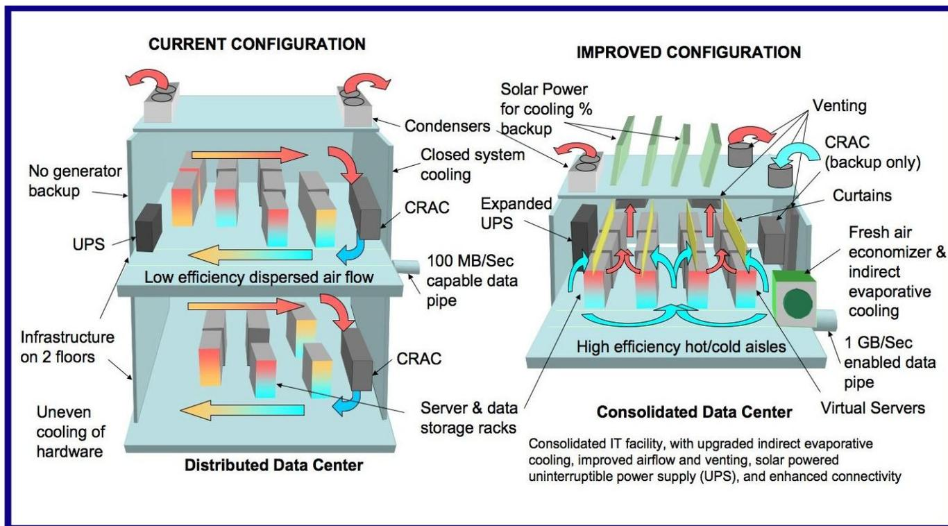
**Figure 6** University of Colorado, Boulder NSIDC data center retrofit: current and improved designs.<sup>6</sup> (Source: Gallaher, David. National Snow and Ice Data Center (NSIDC). University of Colorado, Boulder.)
