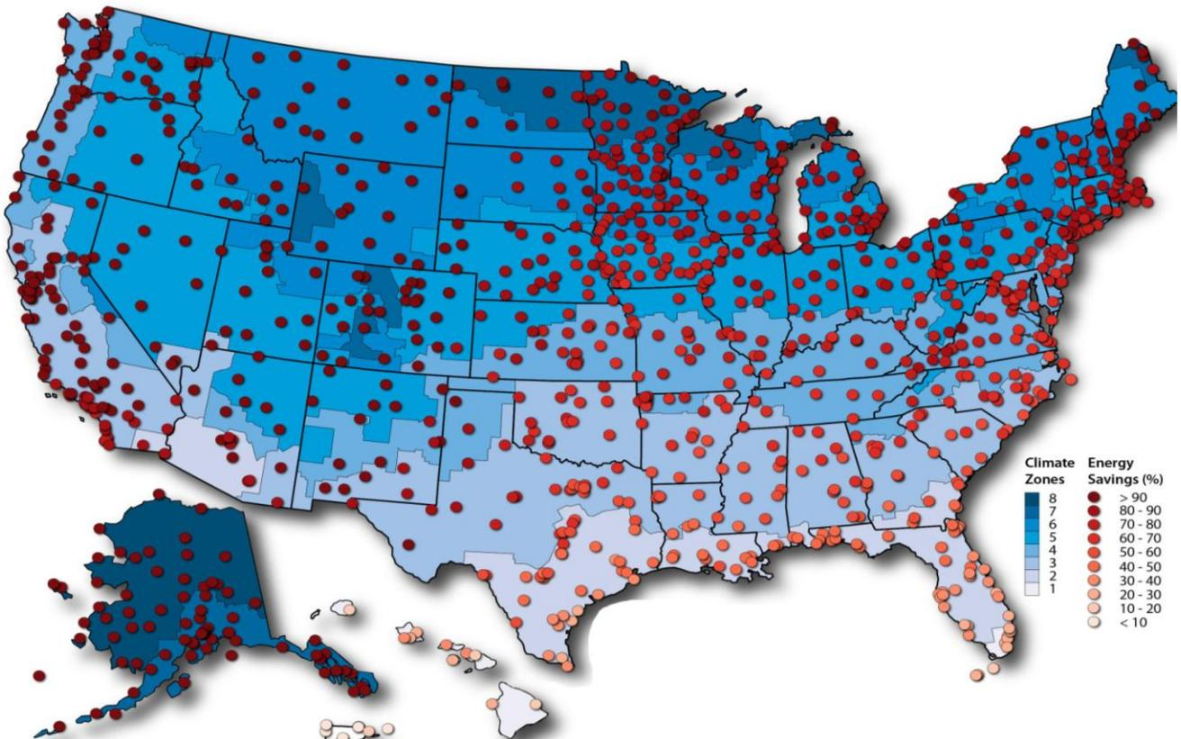
**Figure 5** Energy savings potential for recommended envelope, Stage 3: Economizer + Direct Evap. + Multistage Indirect Evap. Cooling.<sup>15</sup> (Source: Billy Roberts, NREL)
