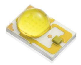
Figure 5-2. Example of the Finished Packaged LED, the Philips Luxeon Rebel
