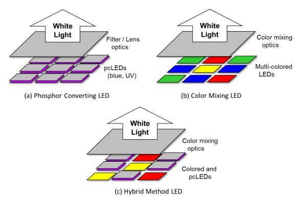
**Figure 4-4. General Types of White Light Emitting Diode (LED) Devices**Source: DOE, 2012b. Solid-State Lighting Research and Development: Multi-Year Program Plan.
