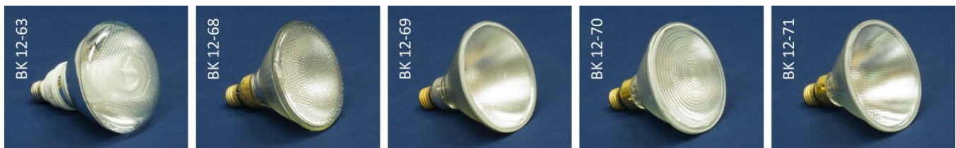
Figure 2. Photographs of five conventional PAR38 lamps (one CFL and four halogen) tested in conjunction with the Series 20 LED products.
