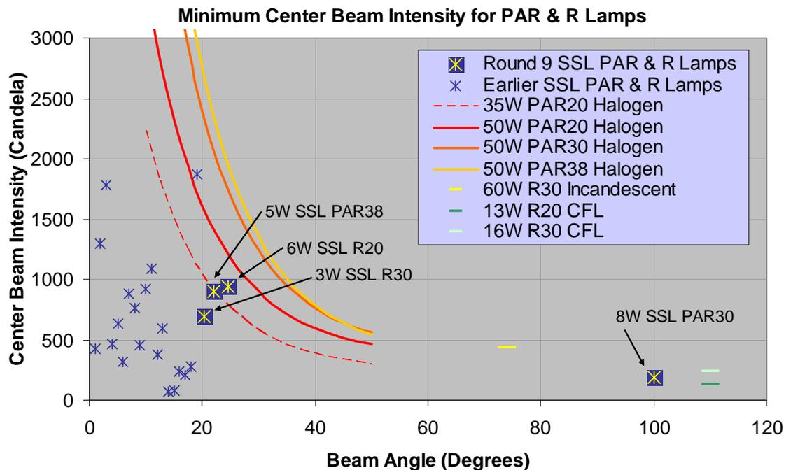
**Figure 8.** Center Beam Intensity for SSL PAR and R Lamps Compared to ENERGY STAR Defined Minimum Center Beam Intensity for Halogen PAR Lamps and Tested Values for Incandescent and CFL R Lamps
