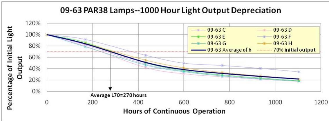
**Figure 10a.** Rapid Light Output Depreciation for SSL PAR38 Lamp
