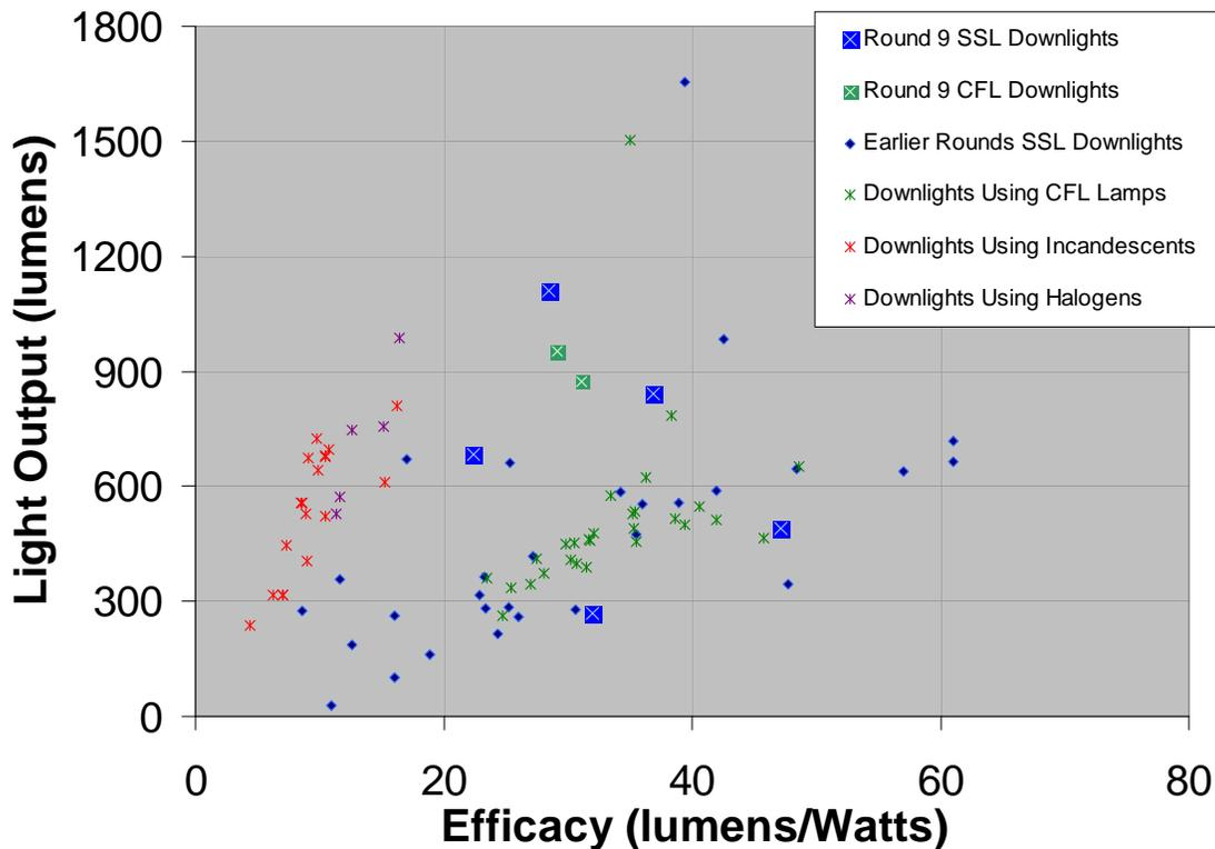
**Figure 2.** Performance of SSL Downlights Compared to Downlights Equipped with CFL, Incandescent, or Halogen Lamps
