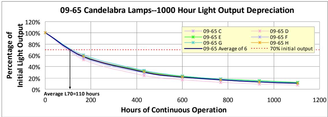
**Figure 10c.** Rapid Light Output Depreciation for SSL Candelabra Lamp
