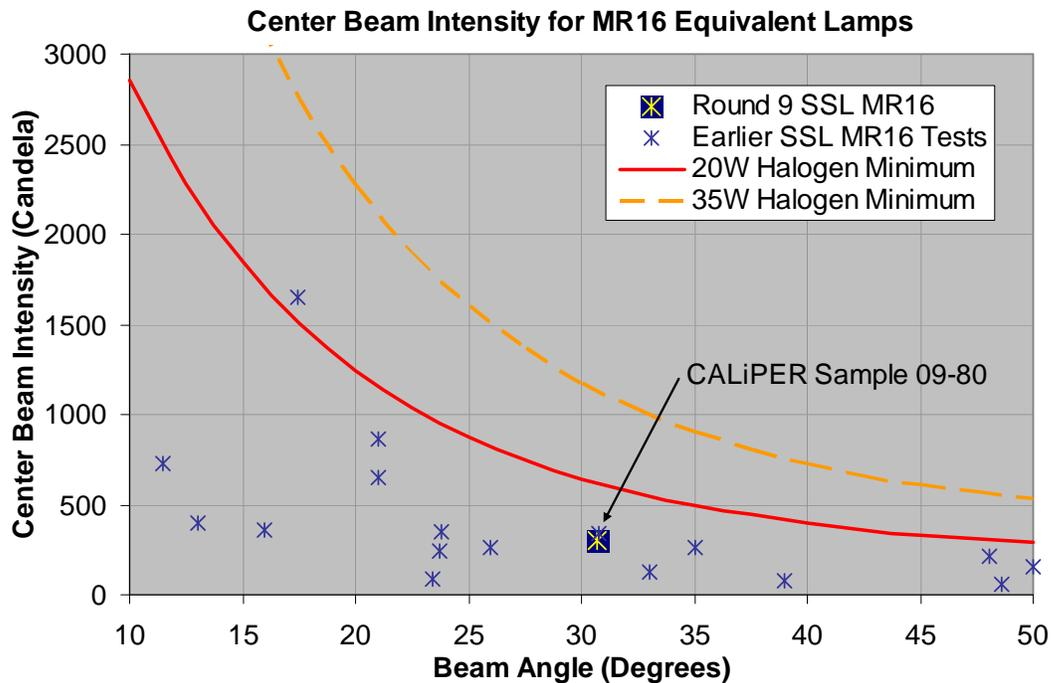
**Figure 7.** Center Beam Intensity for MR16 SSL Lamps Compared to ENERGY STAR Defined Minimum Center Beam Intensity for Halogen MR16 Lamps
