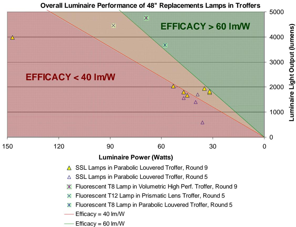
**Figure 3.** Luminaire Light Output and Power for Troffers Equipped with 4’ SSL Replacement Lamps and 4’ Fluorescent Replacement Lamps
