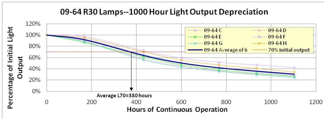
**Figure 10b.** Rapid Light Output Depreciation for SSL R30 Lamp
