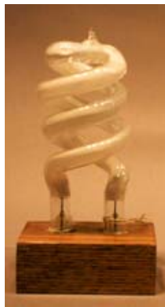
Figure A.2. The "Spiral Lamp" developed by Edward Hammer at GE in 1976. Existing lamp machinery had difficulty making the fragile spiral, and GE felt that new machinery would be too expensive, so they shelved the design. However, spiral lamps appeared on the market in 1995 as other manufacturers decided to see if the design could be competitive. Spiral CFL Smithsonian Institute image #lar2-2d1 {4}
