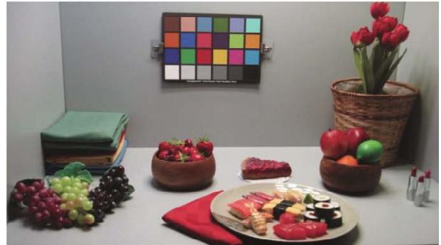
(b) Color-enhancing light ( R_a=71 , Q_a=83 )
