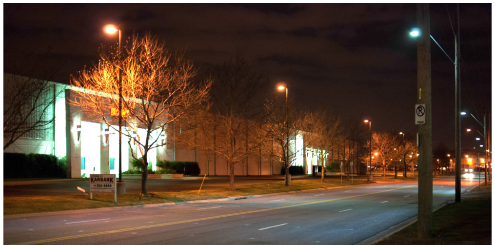
HPS spill light sources and trees potentially causing seasonal variation at one of the Kansas City sites. LED street lighting is at right.
