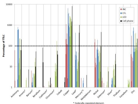
† Some mercury in CFLs is presumed to have escaped detection
