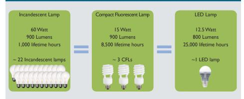
The three lamp types considered in Part 1 are not equivalent in terms of their lumen output and lifetime. So in order to compare apples with apples, 20 million lumen-hours of lighting service was used as a functional unit, with life-cycle energy estimates multiplied by the number of lamps needed to reach this value.
