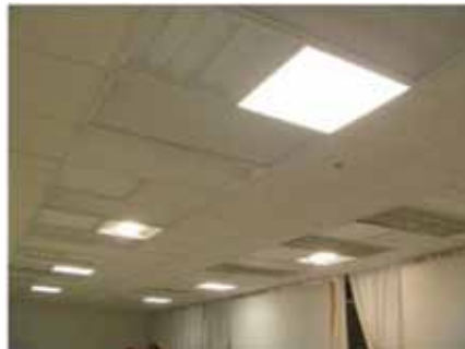
Left: Ceiling of mockup space, showing four sets of 2 ft x 2 ft luminaires spaced on 8 ft x 8 ft centers. Right: Observers evaluating luminaires, using movable wall positioned to show light pattern.
