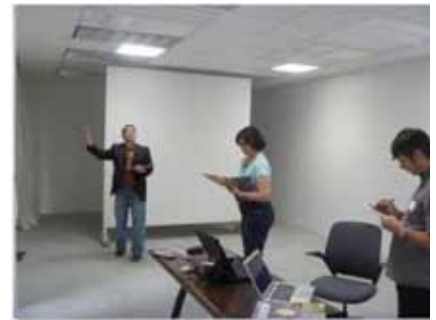
Left: Ceiling of mockup space, showing four sets of 2 ft x 2 ft luminaires spaced on 8 ft x 8 ft centers. Right: Observers evaluating luminaires, using movable wall positioned to show light pattern.
