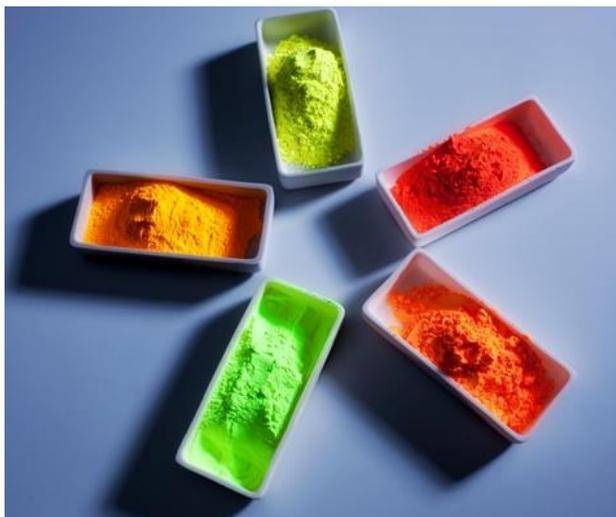
**Figure 2.9 Examples of LED Phosphors**
