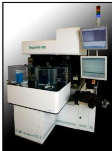
**Figure 2.3 Ultratech Sapphire 100 Stepper for LED Manufacturing**
