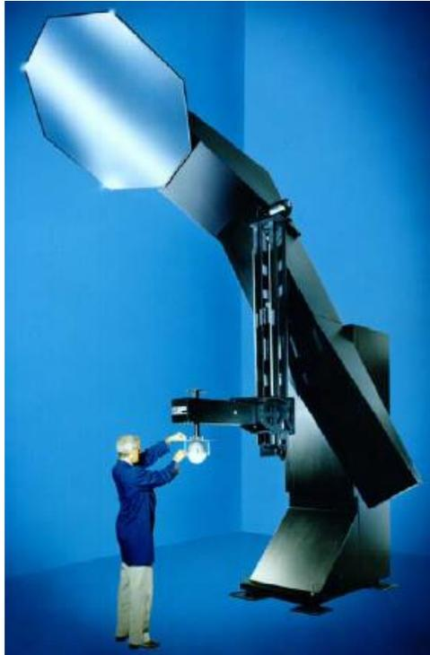
**Figure 2.5 High-Speed Moving Mirror Goniophotometer Model 6400 T**
