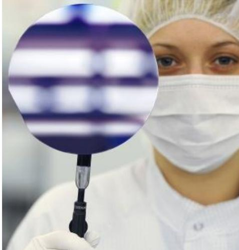
**Figure 2.6 GaN-based LEDs on a 200 mm Silicon Wafer**
