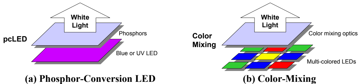
Figure 2-6: General Types of White-Light LED Devices
