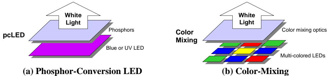
Figure 2-6: General Types of White-Light LED Devices
