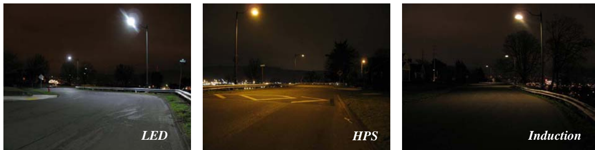
A comparison of visual uniformity from three types of street lighting tested by the City of Portland, Oregon
