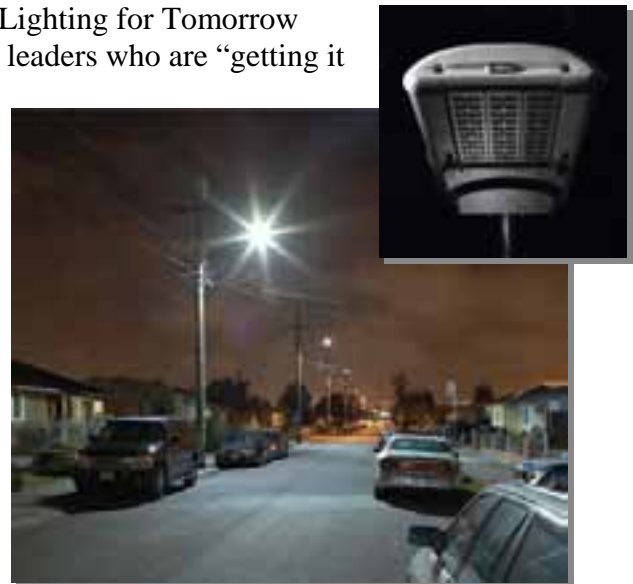
In Phase III of the Oakland demonstration, the installation of next-generation luminaires increased energy savings by 25% and reduced luminaire costs by 34%.
