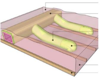
Ducts deeply buried under loose-fill insulation
