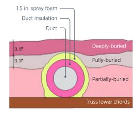
Building America research shows encapsulating the ducts in spray foam before covering with loose-fill insulation provides adequate protection against condensation making this low-cost, high-performance method appropriate for every climate zone.
