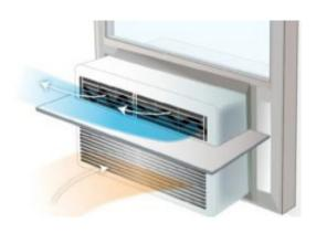
Installing a diverter helps to maximize cool air flow from the air conditioner.
