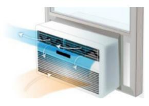
One problem with window air conditioners is that a significant portion of the conditioned air gets recirculated back into the air conditioner.
