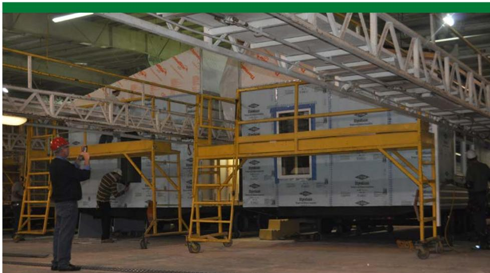
An inch-thick layer of rigid foam wraps around the home. The continuous layer provides insulating, air sealing, and drainage plane in one step, eliminating the need for house wrap and taking the place of OSB or plywood sheathing for considerable time and cost savings. The foam layers stop heat transfer through the studs, boosting the wall's overall thermal performance.
