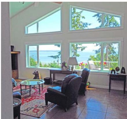
The stained concrete floors provide thermal mass while triple-pane windows let in sun for passive solar heating.
