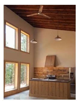
The stained concrete flooring is durable and moisture resistant. The floor's thermal mass serves as a heat sink to help moderate indoor temperatures.
