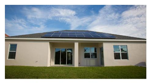
The home's 6.84-kW photovoltaic power system provides enough energy to power the home and an electric car.
