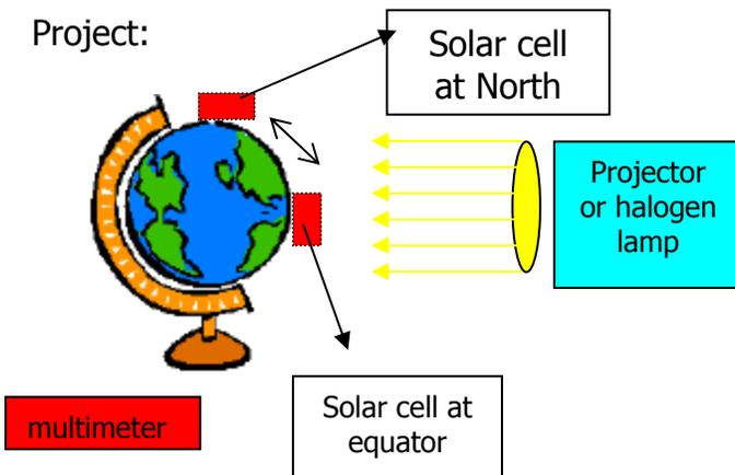
**Materials and Equipment:** World globe or Styrofoam sphere, solar cell and/or pyranometer, multimeter, Velcro tape, protractor/angle finder, projector and/or halogen lamp.
