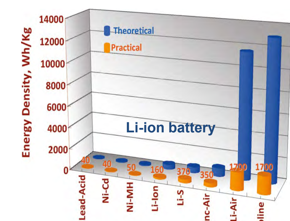
Figure 1 The gravimetric energy densities (Wh/kg) for various types of rechargeable batteries compared to gasoline.
