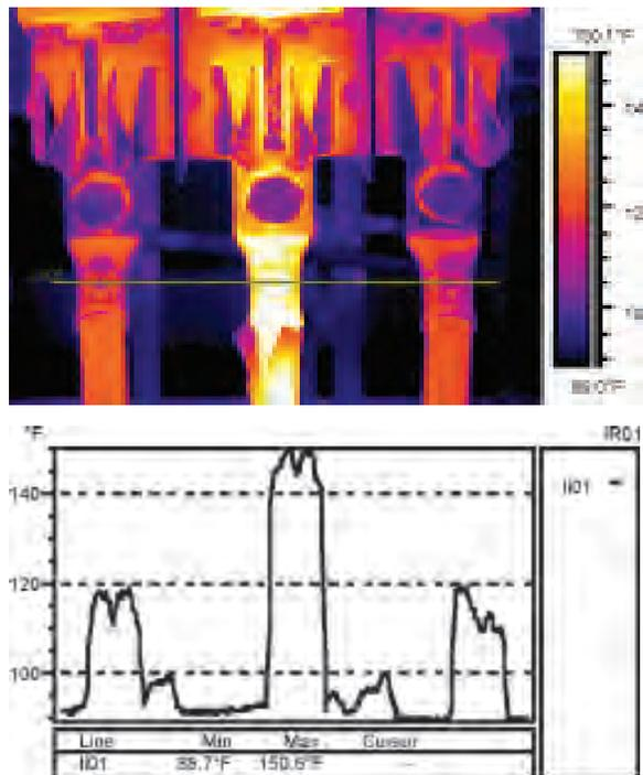
Software analysis tools can quantify and graphically display temperature data. As shown above, the middle conductor/connection is a much higher temperature indicating a loose connection.
