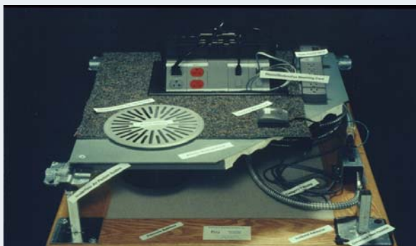
Components within the SCROB's Raised Floor System
