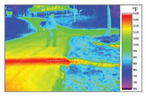
**Figure 6.2.12**. Steam or hot water distribution system leaks and/or underground line location can be defined with IR.
