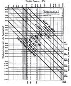
Figure 6.5.1. Vibration severity chart
