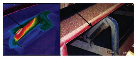
**Figure 6.2.8**. Seized conveyer belt roller as indicated by elevated temperatures in belt/roller contact area.
