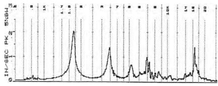
**Figure 6.5.2**. FFT – Example of graph breaking down vibration level at different frequencies
