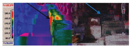
Figure 6.2.6. IR scans of multiple electric motors can highlight those with hot bearings indicting an imbalance or wear problem.
