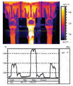
Software analysis tools can quantify and graphically display temperature data. As shown above, the middle conductor/connection is a much higher temperature indicating a loose connection.
