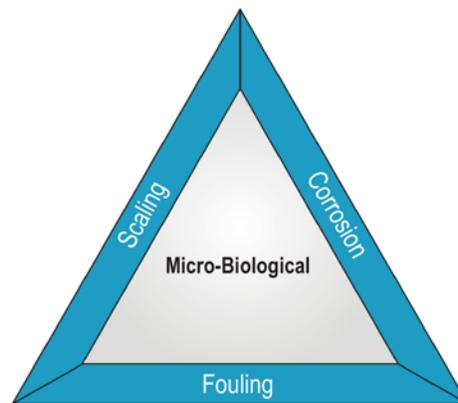
**Figure 1.1. Cooling Tower Primary Treatment Concerns.**
