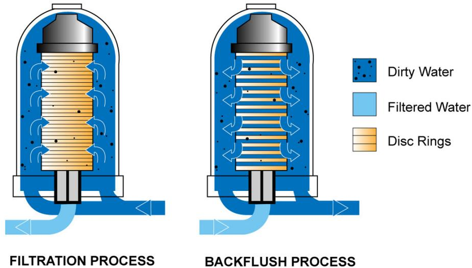
**Figure 2.3. Plastic Disc Filters.**
