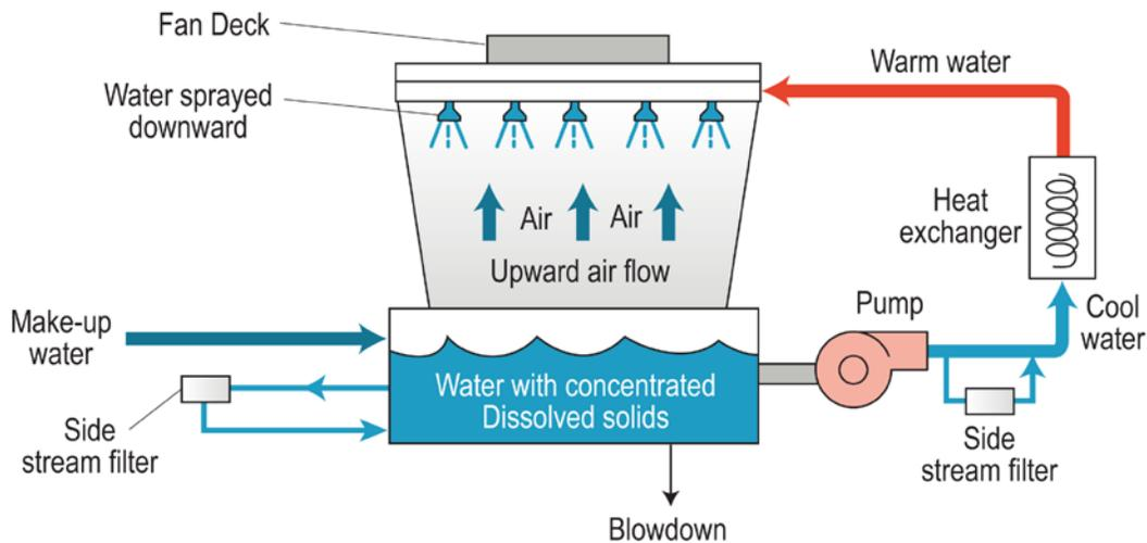
Figure 1.2. Cooling Tower with Side Stream Filtration Examples.
