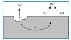
Figure 7. Example of a Corrosion Cell.
