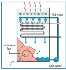
Figure 1. Example of a Closed Circuit Cooling Tower.
