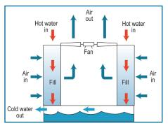
Figure 6. Example Cross-flow Cooling Tower.
