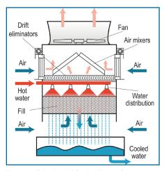
Figure 2. Overview of Cooling Tower Structure Components.
