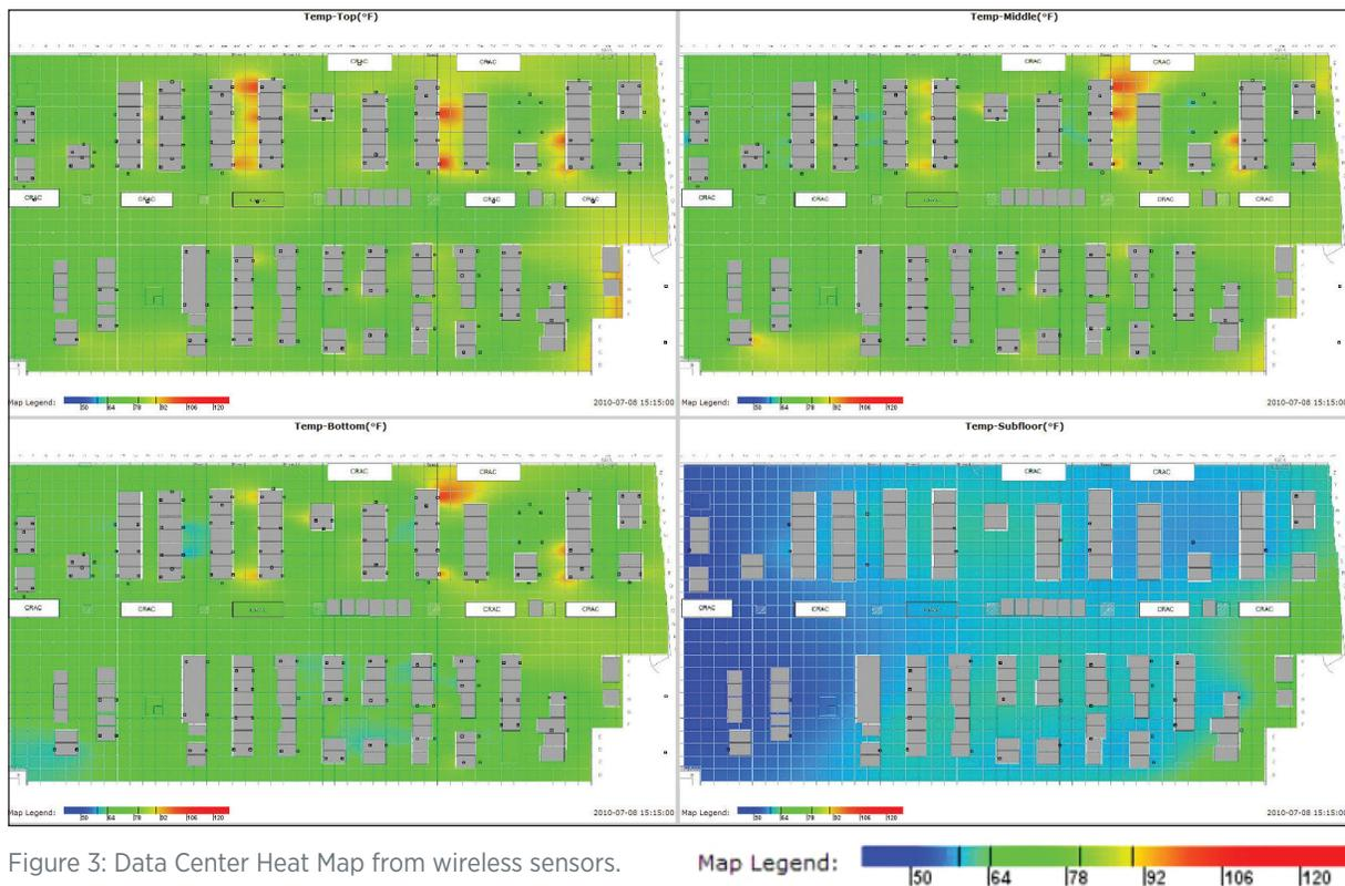
Figure 3: Data Center Heat Map from wireless sensors. Courtesy: SynapSense Corp.
