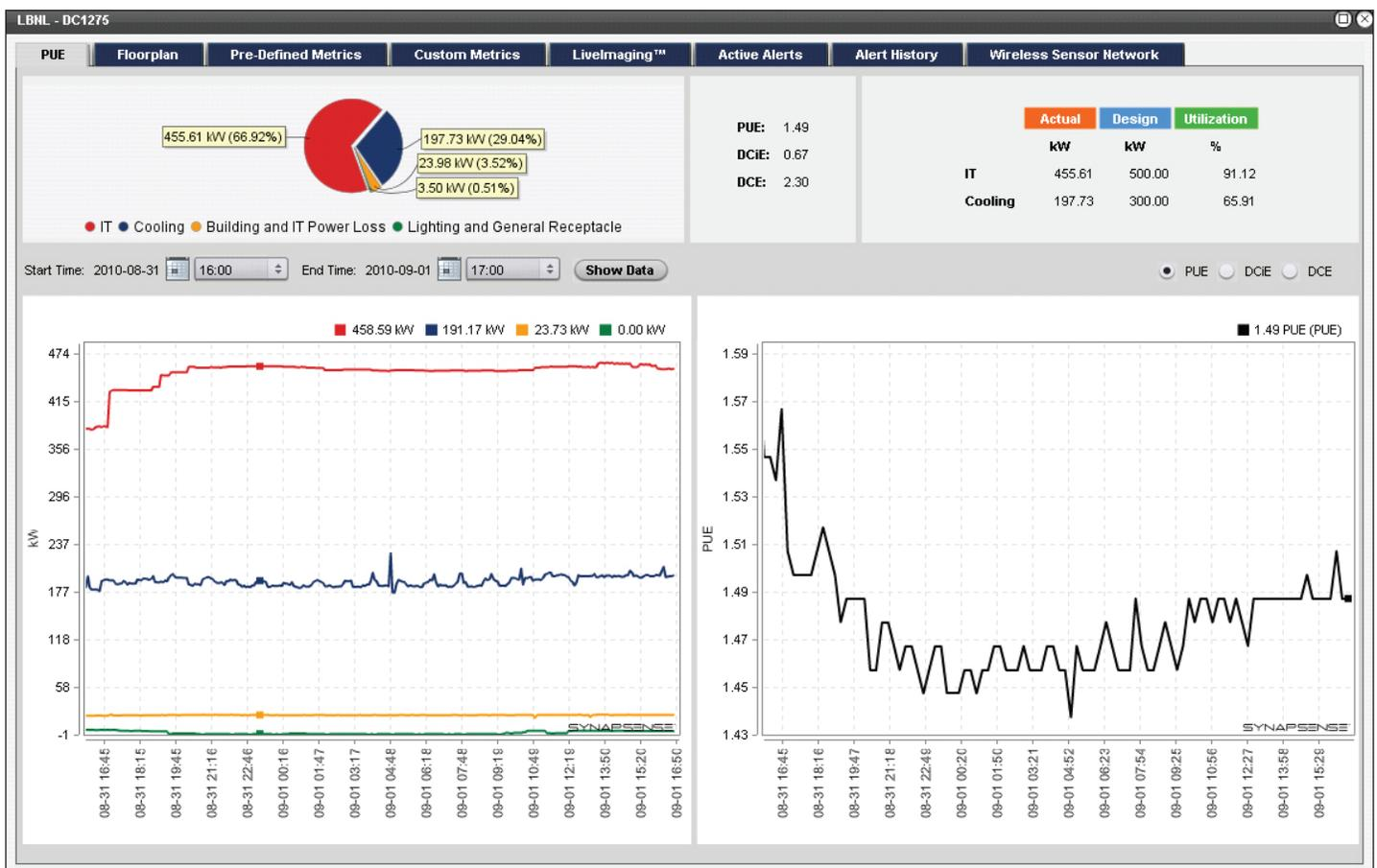
Figure 11: Calculated Real-time PUE. Courtesy: SynapSense Corp.
