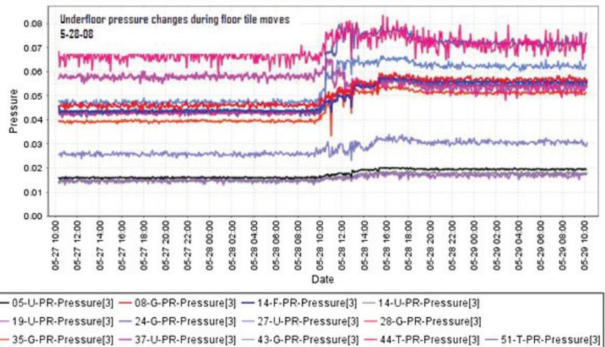
Figure 5: Under-floor pressure improvement from floor-tile tuning.
